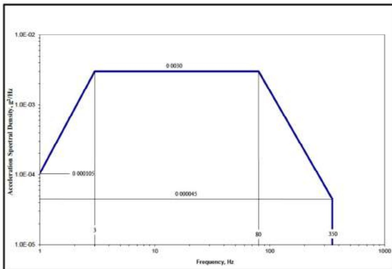
Figure 514.8C-17. Category 11 - Rail cargo vibration exposure.
