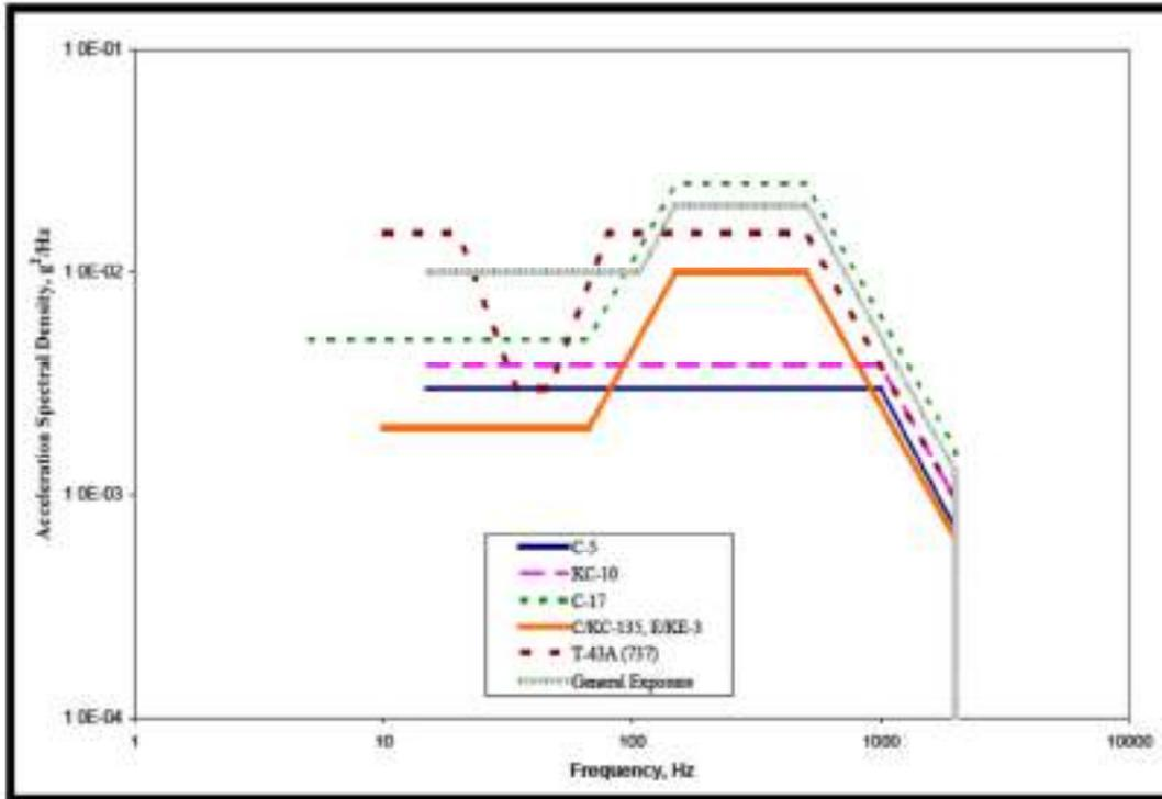
Figure 514.8C-9. Category 7 - Jet aircraft cargo vibration exposure.
