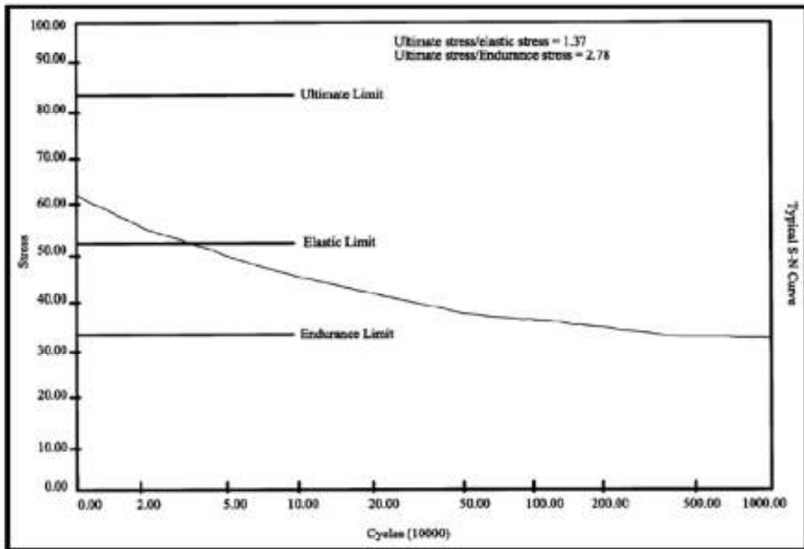
Figure 515.8F-6. Typical S/N curve.
