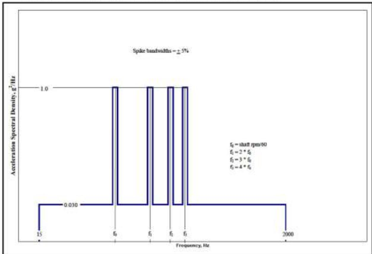
Figure 514.8D-12. Category 22 - Turbine engine vibration exposure.
