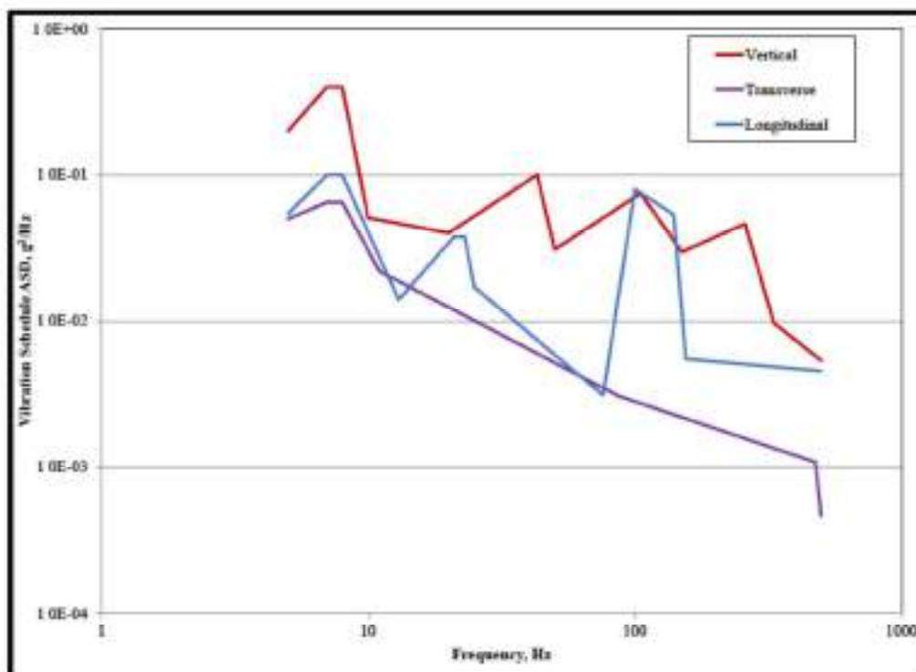
Figure 514.8C-4. – Category 4 – Composite two-wheeled trailer vibration exposure.
