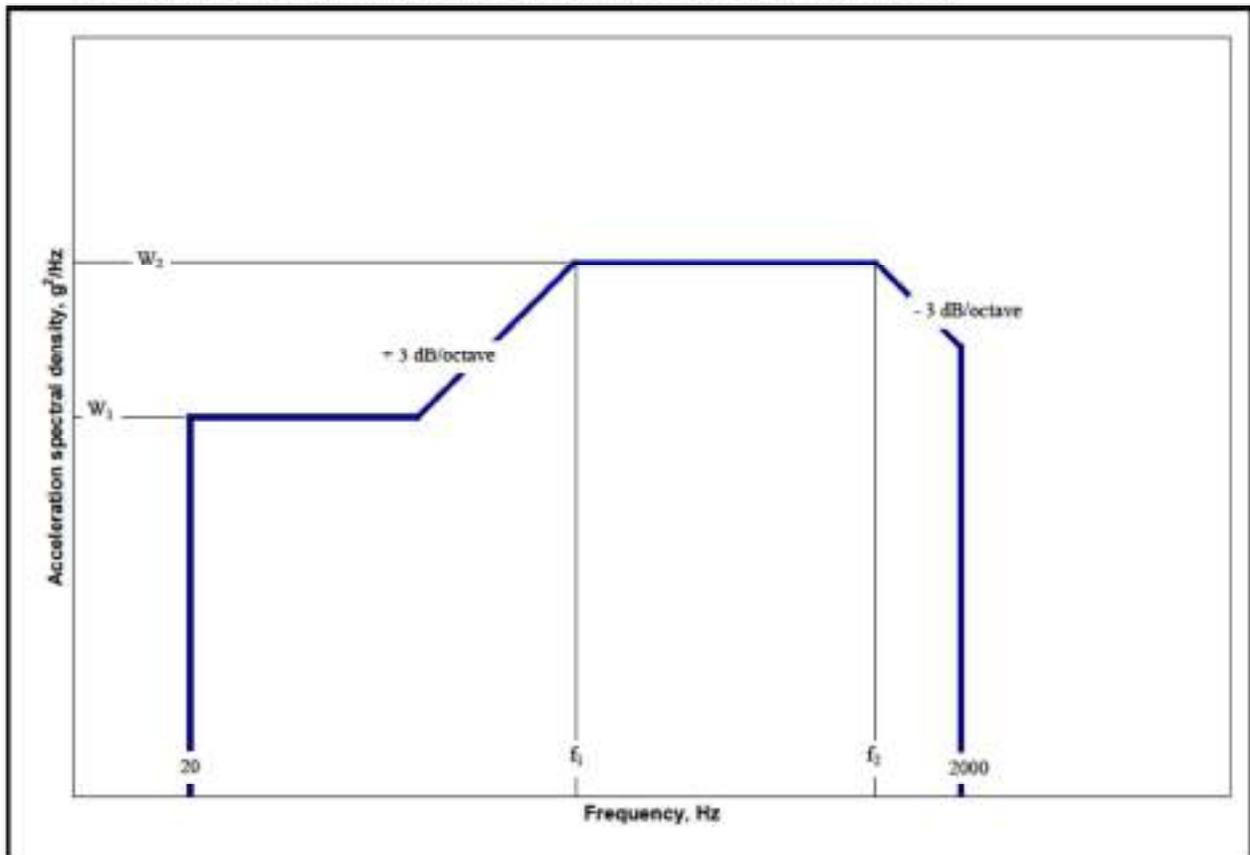
**Figure 514.8D-9. Category 16 - Jet aircraft store equipment vibration exposure.**
