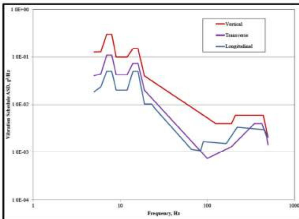
Figure 514.8C-6. – Category 4 – Composite wheeled vehicle vibration exposure.
