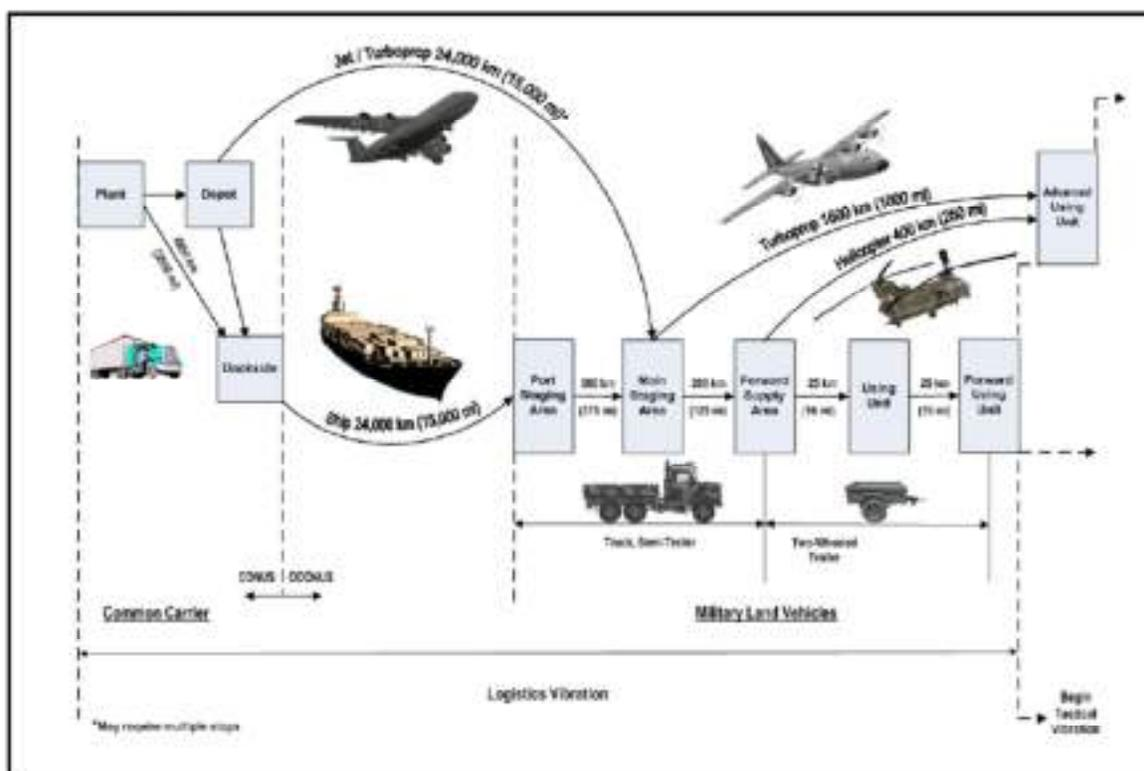
Figure 514.8C-1. Typical mission / field transportation scenario.<sup>1,2</sup><sup>1</sup>See paragraph 6.1, reference na.<sup>2</sup>In the event that tracked vehicles are identified in LCEP, they should be considered in the typical mission/field transportation scenario. See paragraph 6.1, reference d.
