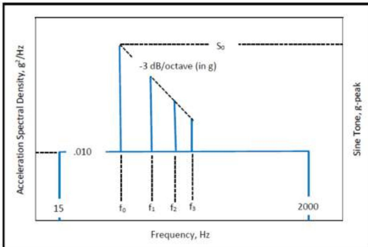
Figure 514.8D-2. Category 13 - Propeller aircraft vibration exposure.
