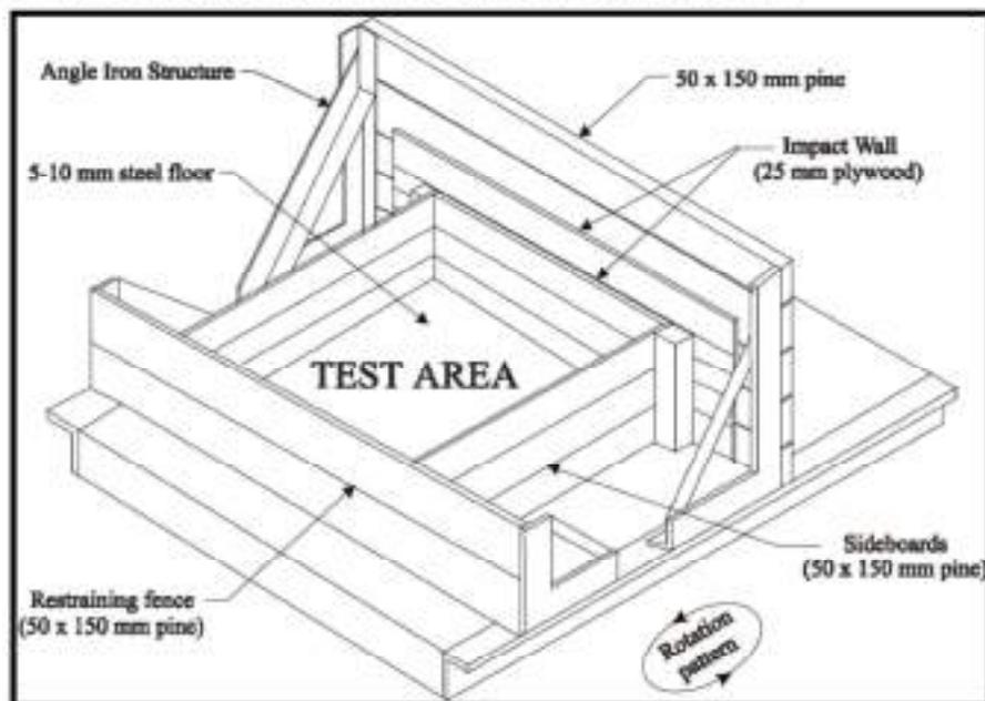
Figure 514.8C-8. Category 5 - Loose cargo test setup.
