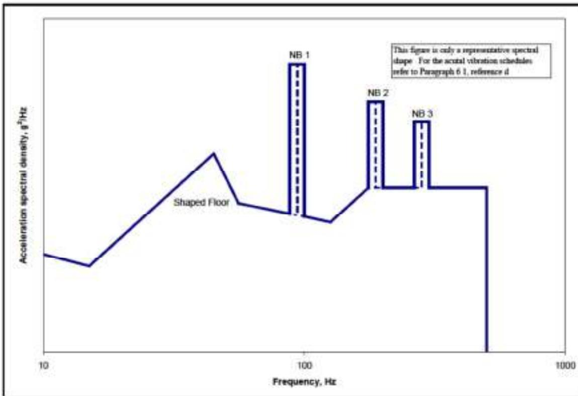
Figure 514.8D-10. Category 20 - Tracked vehicle representative spectral shape.
