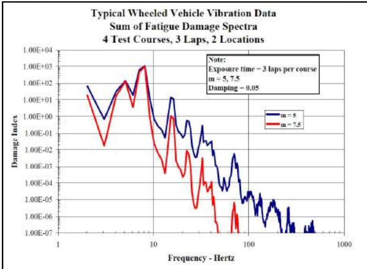
Figure 514.8F-C.6. Fatigue damage spectra for two exponents.
