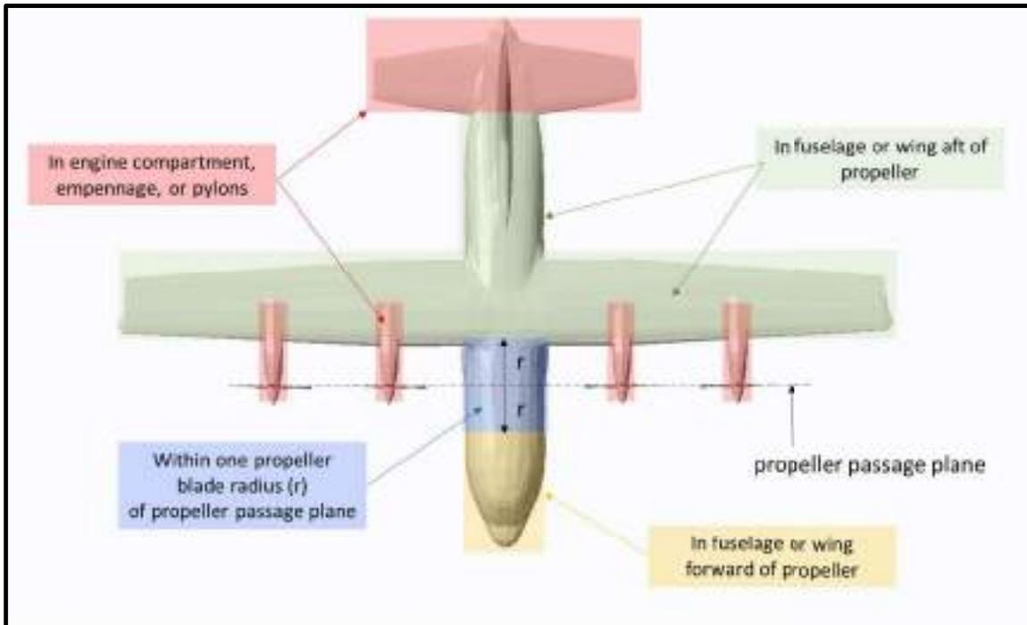
Figure 514.8D-3. Category 13 - Propeller aircraft installed equipment locations.
