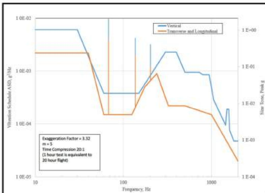
Figure 514.8C-11. Category 8 - Propeller aircraft vibration exposure, 4-bladed C-130.
